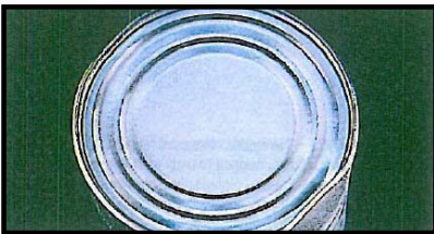
Figure 6: Minor dent to double seam on end of can body, i.e., it does not appear creased or sharp.
